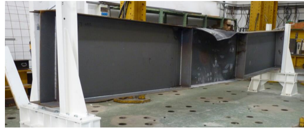
Local buckling for flange 300 mm x 8 mm
