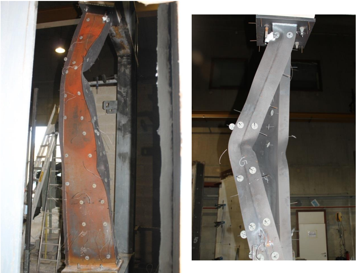
Figure 105: Deformed shape after test 4
