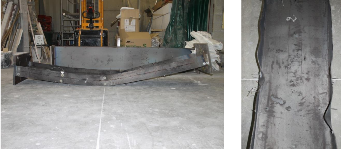
Figure 101: Deformed shape after test 2
