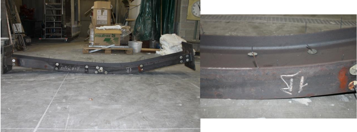
Figure 99: Deformed shape after test 1
