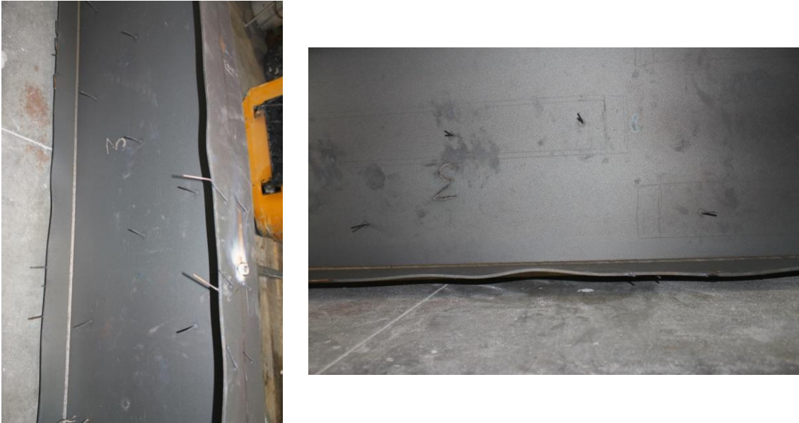
Figure 103: Deformed shape after test 3
