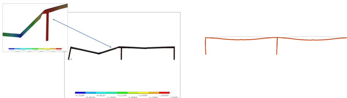
Figure 158: Failure mode for internal column fire: left) shell model, right) new beam element model
