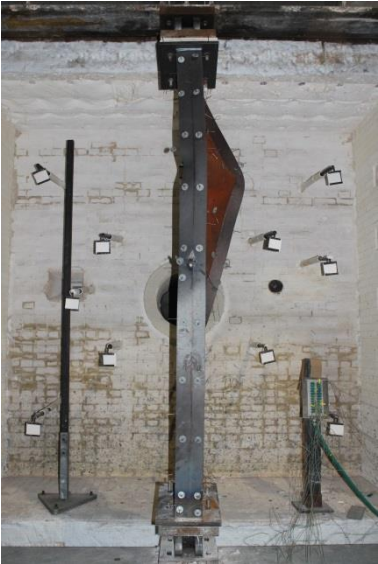
Figure 6: illustration of the global buckling of the tapered column (small cross-section at top)
