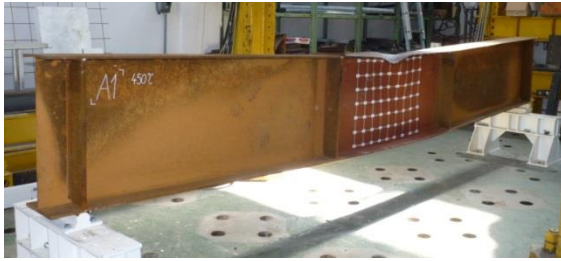
Local buckling for flange 250 mm x 12 mm
