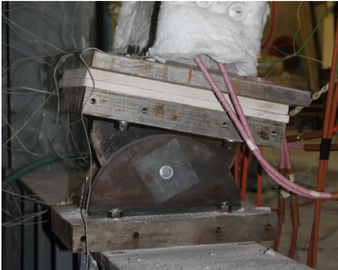
Figure 95: Pinned support with thermal disconnection
